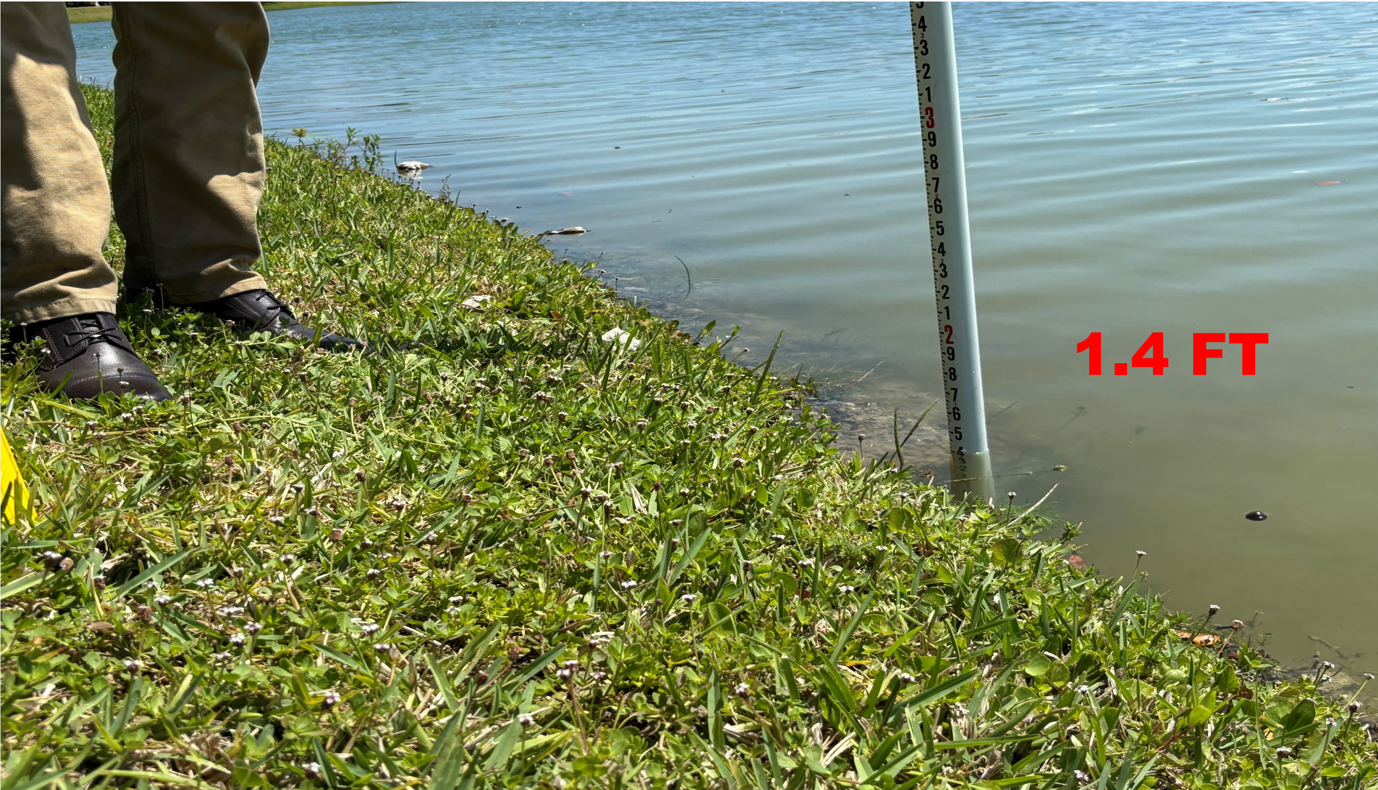
1.4 FT VERTICAL EROSION - MAY WATER LEVEL
