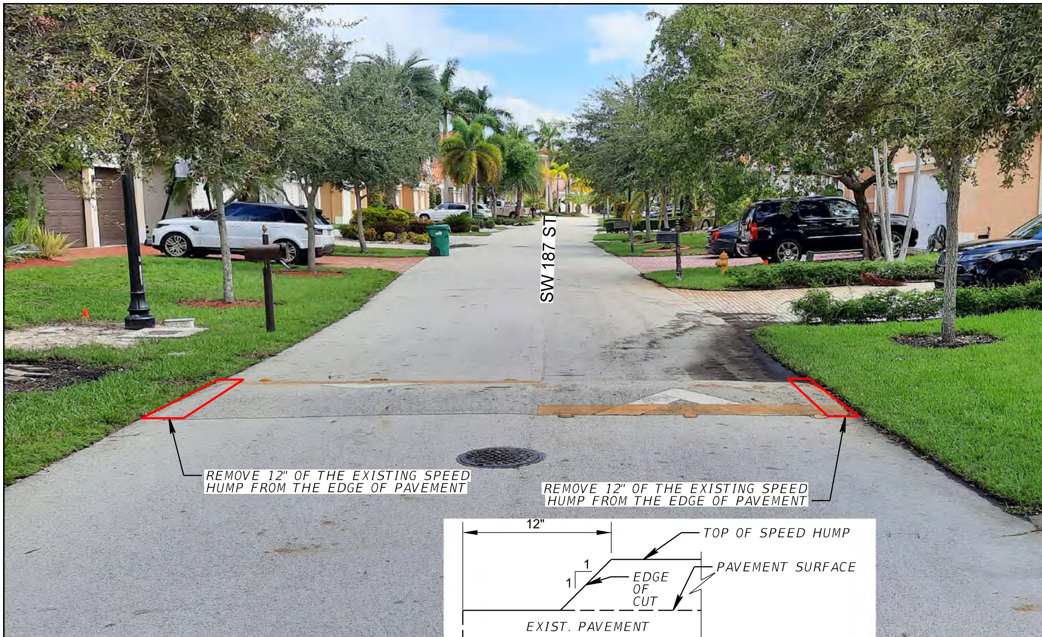
SPEED HUMP REMOVAL DETAIL (TYPICAL) (NTS)
